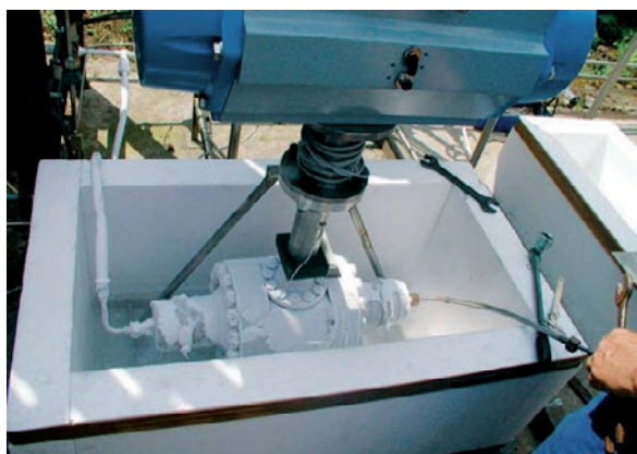
Cryogenic testing – ball valve NPS 4 CLASS 600
