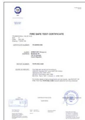
Certyfikat FIRE SAFE ISO 10497, API Standard 607 / FIRE SAFE Certificate acc. to ISO 10497 and API standard 607
